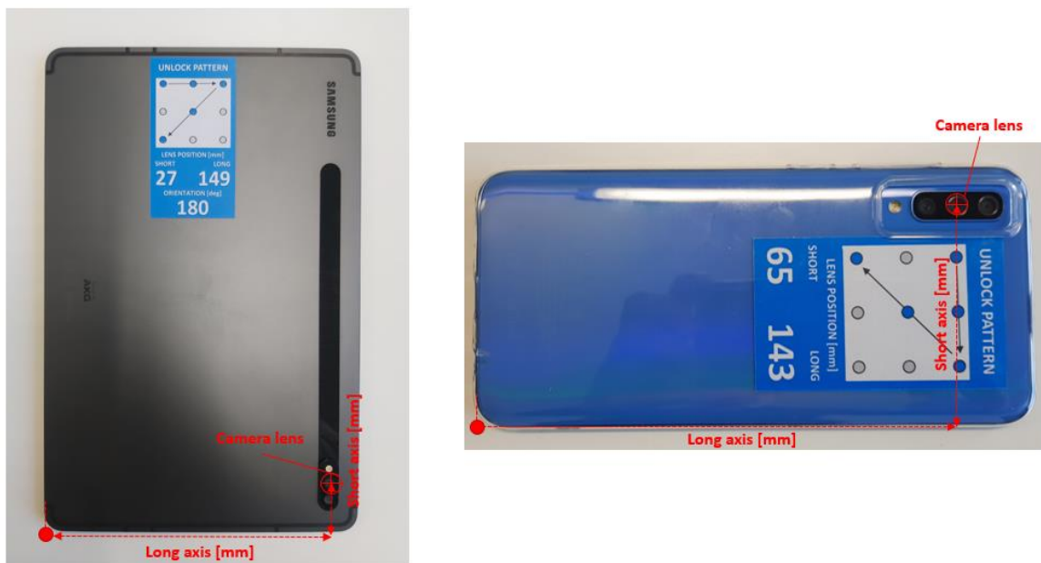
Figure 6 Determine the values for the short / long axis of the camera lens position (tablet on the left, smartphone on the right)
