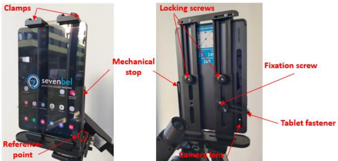
Figure 19 Insert the Tablet and verify its orientation.
