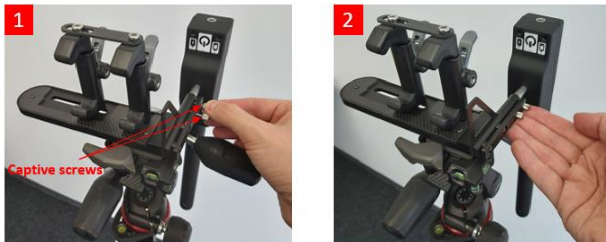
Figure 13 Fasten the captive screws to secure the position of the sensor.
