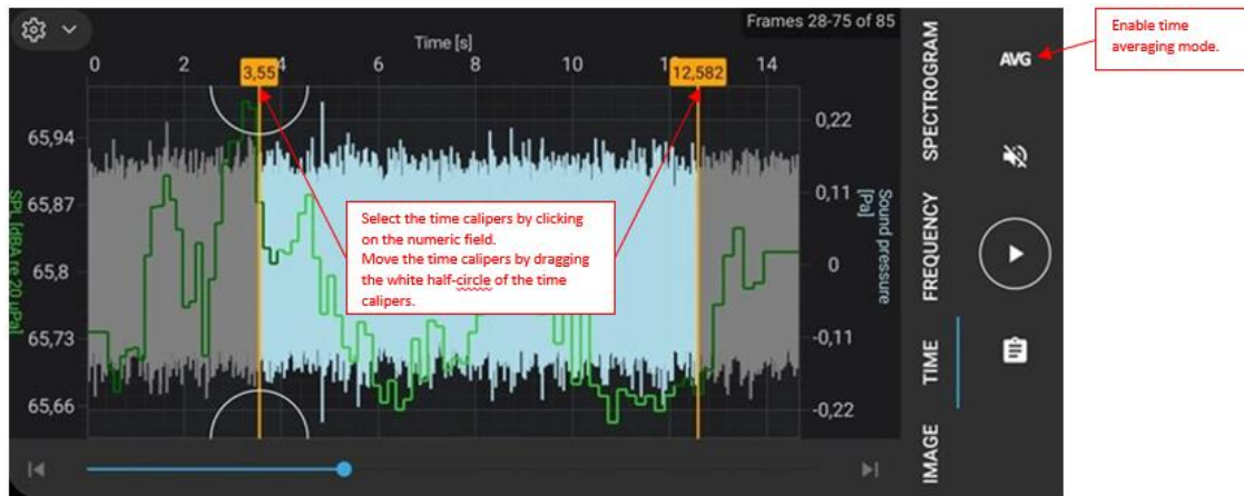
Figure 38 Audio signal of the reference microphone at the center of the sensor for the currently selected averaged acoustic image.
