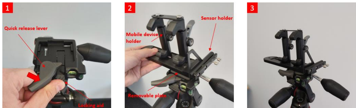
Figure 11 Mounting the sensor holder.
